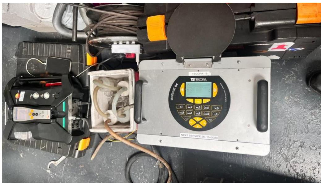
Figure 1: Yellow Tree's Emissions Sampling Equipment at Flaura Pets
